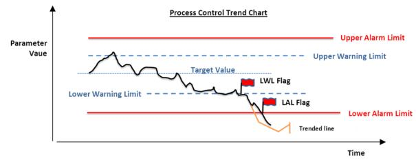
**Figure 4 - Typical Process Control Trend Chart**
